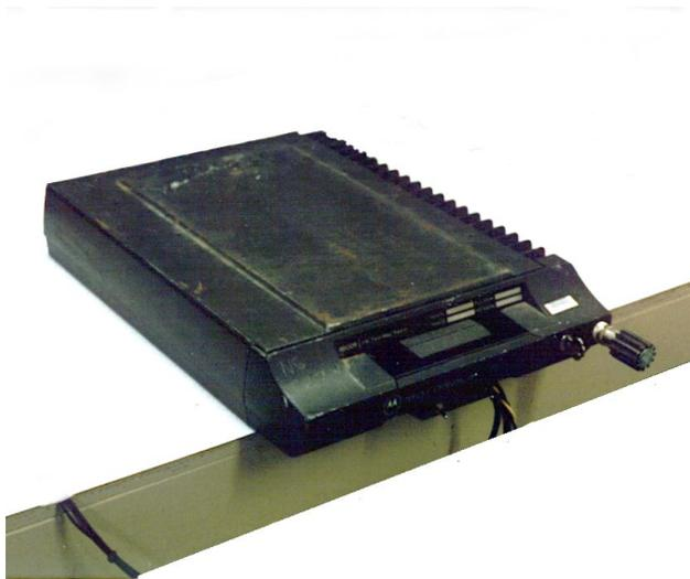
The transmitter employs a heterodyne exciter. Receiver oscillator injection is mixed with the signal from an offset oscillator to generate the transmit frequency. The offset oscillator is varactor modulated for true FM.
