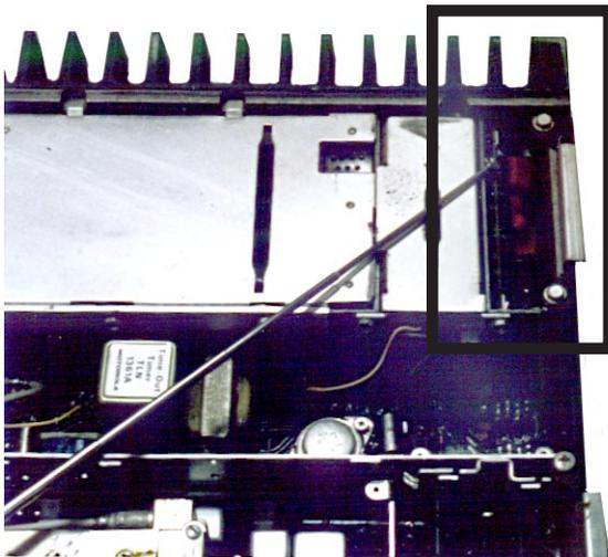
3. Remove the audio-squelch board. This board is held in place by 4 screws and is removed from the top side of the radio.
