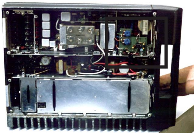
Picture of Perf Board for TPRS Modem modification. Mounted in Upper Right Corner.
