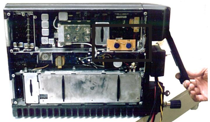
Picture of Perf Board for TAPR/G3RUH Modem modification. Mounted in Upper Right Corner.
