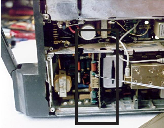
2. Remove the TX PL encoder (if installed). This board plugs into the exciter board from the bottom side of the radio. The encoder board location is also shown in the bottom view of the radio.
