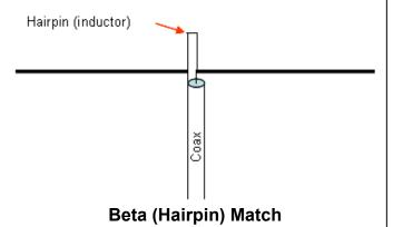
the driven element, in reality the hairpin has some inductance, and this inductance is in parallel with the feedpoint input. The hairpin requires that the feedpoint impedance be less than 50 ohms, and that it exhibit a capacitive series reactance (driven element is a bit short).
