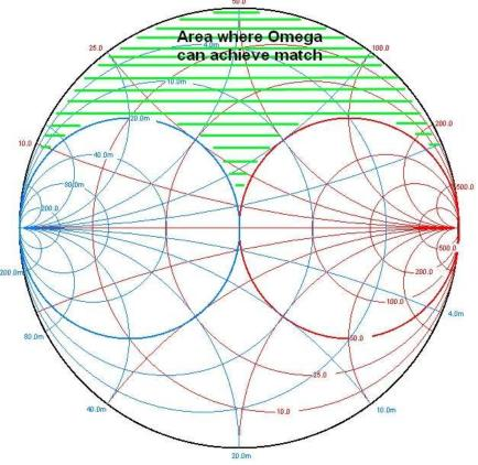
The range of input impedances presented by the gamma rod that can be matched to 50 ohms with an omega match is the green shaded area in the upper portion of the chart.
