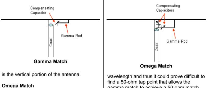
wavelength and thus it could prove difficult to find a 50-ohm tap point that allows the gamma match to achieve a 50-ohm match. In this case, an additional variable capacitor can be added to substantially increase the range over which the match can be
