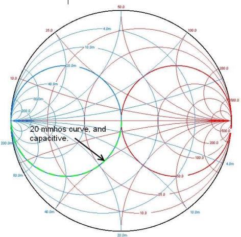
The range of input impedances that can be matched to 50 ohms with a hairpin (beta) match is the half-arc shown by the dashed green line.
