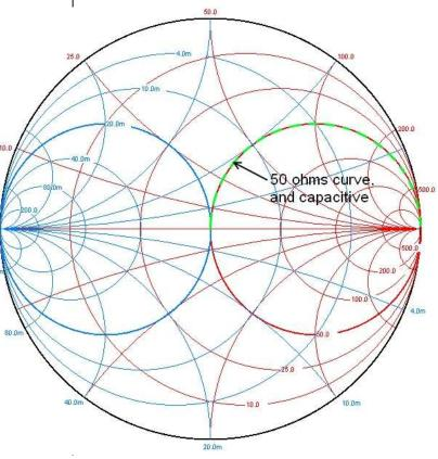
The range of input impedances that can be matched to 50 ohms with a gamma match is the half-arc shown by the dashed green line.
