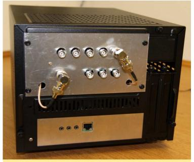
Back of the radio showing multiple Antenna connectors, Microphone, CW Key, Speaker, and Ethernet Connectors.
