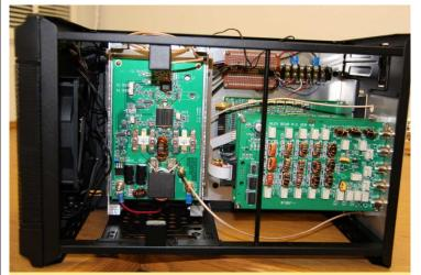
Top view. 100w amplifier left, filters right.
