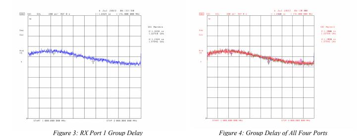
The propagation delay through all four channels is virtually identical: about 1.28 nanoseconds at L5, 1.31 ns at L2, and 1.16 ns at L5. Because there is no filtering to introduce additional delays, the GUS adds very little electrical length to the cable.
