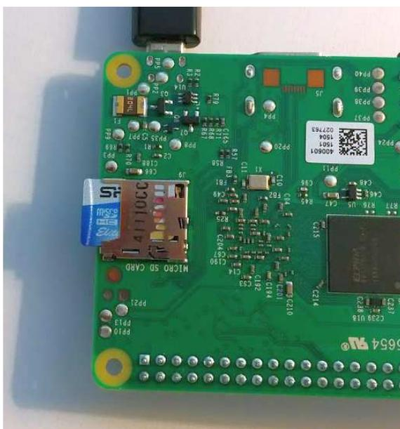
*Figure 3: SD Card Inserted into rPi*
