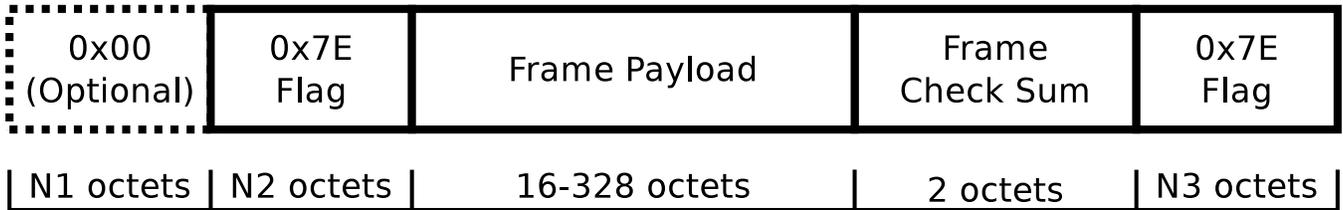
Figure 3: Amateur Bell 202/HDLC frame format
