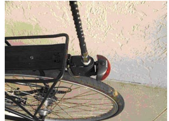
Figure 3. Hamstick mounted to rear carrier with angle bracket.
