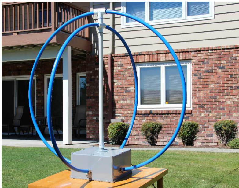
Figure 10 - Homebrew dual active-loop receive antenna (vertically polarized). Only one of the two loops is used in this experiment.
